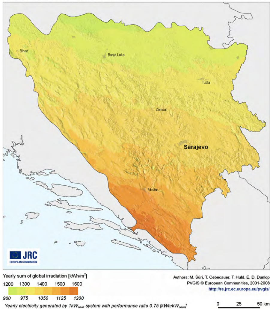
Fig. 2. Yearly sum of total solar irradiation incident on horizontal PV modules in kWh/m 2 and yearly electricity generated by 1 kWp system with performance ratio 0.75 (kWh/kWp) for the territory of Bosnia and Herzegovina obtained by PVGIS. Adapted for Bosnia and Herzegovina from PVGIS©European Communities, 2001–2008, http://re.ec.europa.eu/pvgis/ .
