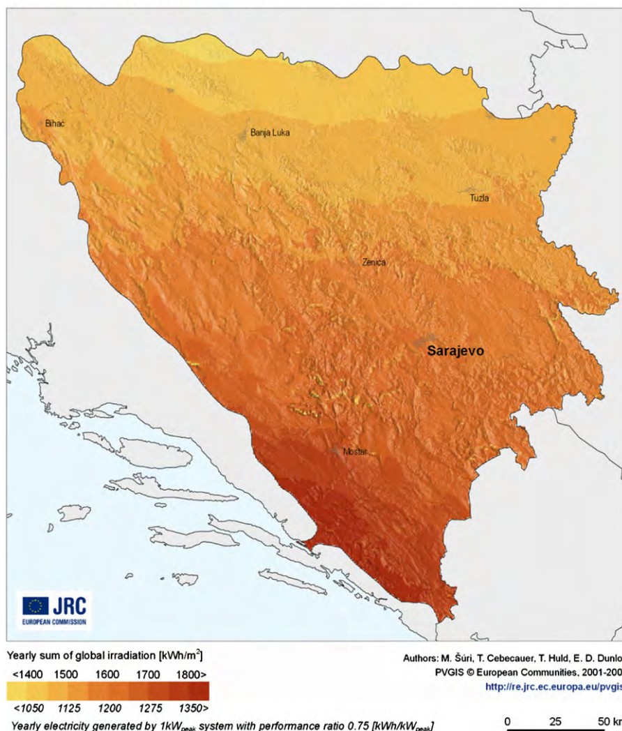
Fig. 3. Yearly sum of total solar irradiation incident on optimally inclined south-oriented PV modules in kWh/m 2 and yearly electricity generated by 1 kWp system for the territory of Bosnia and Herzegovina obtained by PVGIS. Adapted for Bosnia and Herzegovina from PVGIS © European Communities, 2001–2008, http://re.ec.europa.eu/pvgis/ .
