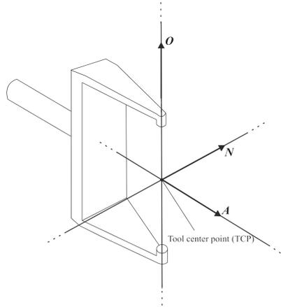
**Figure 4** The dual tool frame of a robot end-effector.
