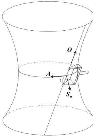
**Figure 5** A robot end-effector which moves on the surface of a right circular hyperboloid of one sheet.
