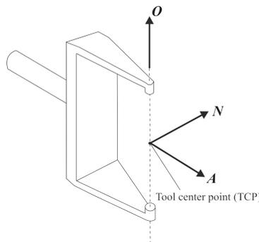
Figure 1 A robot end-effector and its tool frame.
