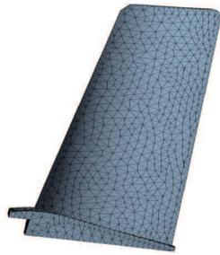
Figure 2 The FEM of blade
