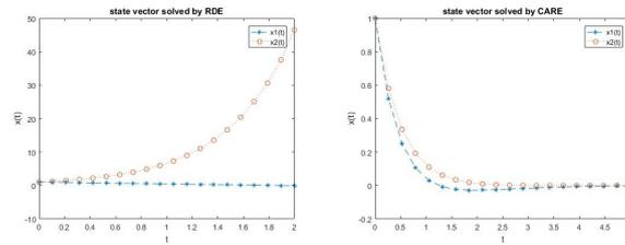
Figure 1: Continuous-Time System: State vectors solved by RDE (Left) and CARE (Right)
