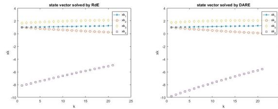
Figure 2: Discrete-Time System: State vectors solved by RdE (Left) and DARE (Right)
