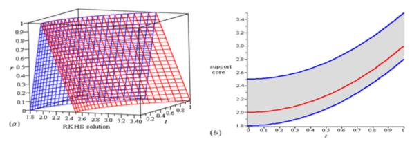
**Figure 1**: Geometric behavior for fuzzy approximate solution of Example 5.2 **(a)** The RK solution in terms of *r*-cut representation form (blue is the left branch solution; red is the right branch solution) **(b)** The support and the core of the RK solution (gray is support and red is core).
