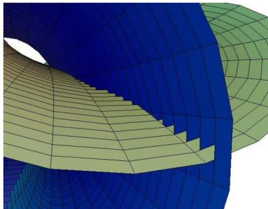
Figure 1: Intersection of surfaces in polygon mesh
