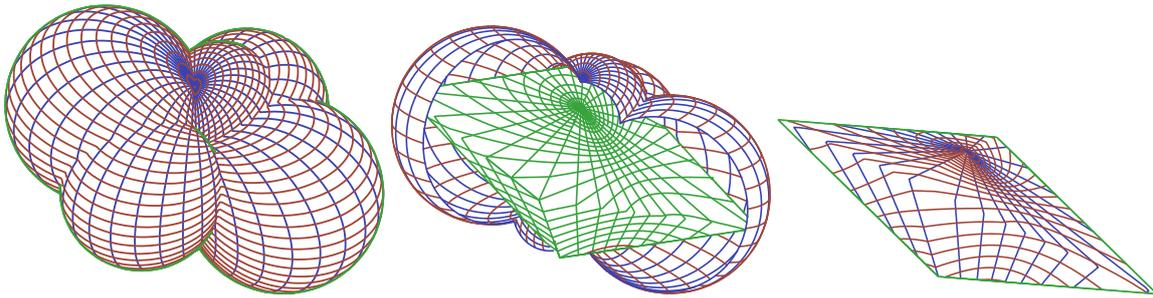
Figure 13: Potential surface and the corresponding Wulff's crystal
