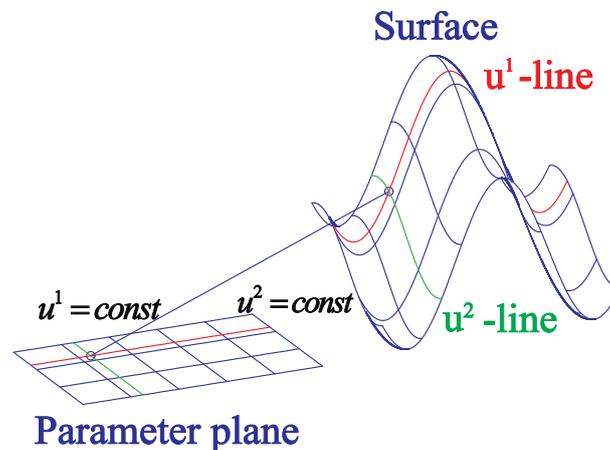
Figure 3: Parameter lines on a surface
