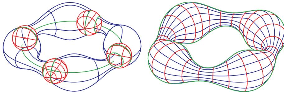
Figure 7: A tubular surface as the envelope of spheres; concept (left), reality (right).
