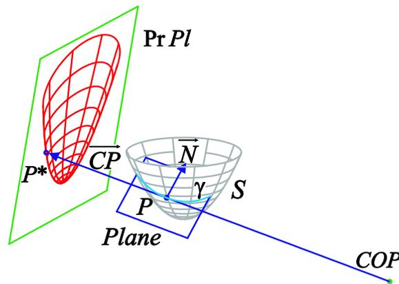
Figure 9: The definition of a contour point of a surface
