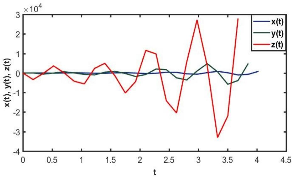
Figure 13: the instability behaviour for (2.14) with  $h = 0.18$  and  $\sigma = 0.5$
